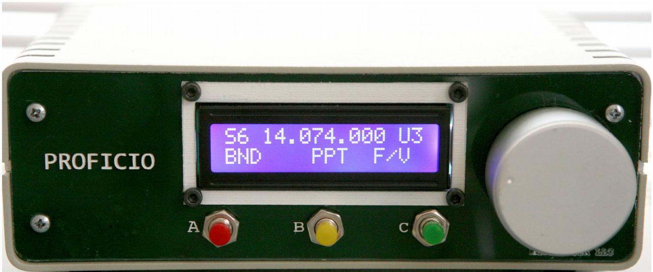
The top line of the display displays an S Meter value, the frequency, the mode of operation and the frequency step increment.
